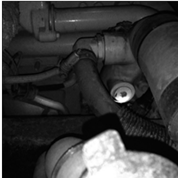
Figure 4: Location of coolant return plug
