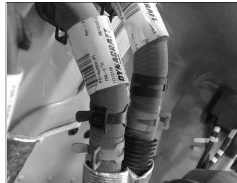
Figure 20: Cab heater circuit
