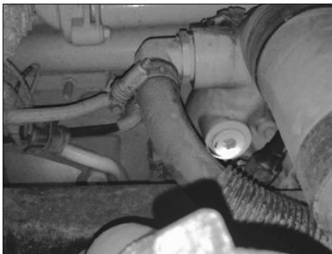
Figure 18: Location of coolant return plug
