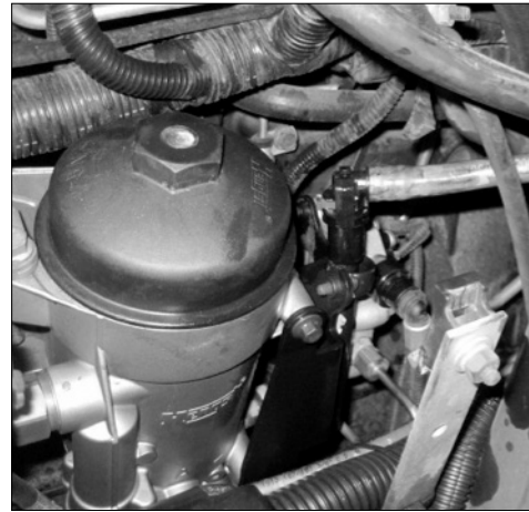
Figure 12: Re-route Return Fuel Line
