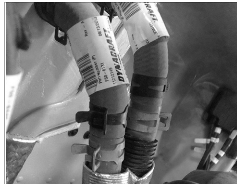
Figure 20: Cab heater circuit
