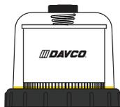
When new, the fuel level in the filter will be very low with minimal restriction. As the filter is used, contaminants collect on the filter from the bottom up. Fuel rises on the filter indicating remaining filter life.
