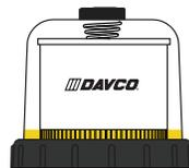
Fuel level increases in clear cover. As contaminants collect on the filter, the fuel rises to a non-contaminated section of the filter, providing optimal filtration while maintaining lowest restriction.
