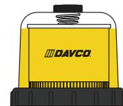
The filter element is now completely covered by fuel. At this point, all of the media's surface area is utilized. Restriction is increasing and the filter element should be changed at the next scheduled maintenance interval.
