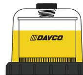
Fuel level at filter wrap level. Even though the fuel level is now more than half of the filter element, the fuel is still flowing through clean media at minimal restriction levels. The filter still has significant life remaining.
