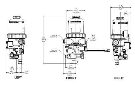
Mounting Hole Distance: [150] Mounting Hole Openings: [11]
