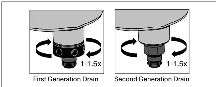
3. Using the Collar Wrench, loosen the collar.
