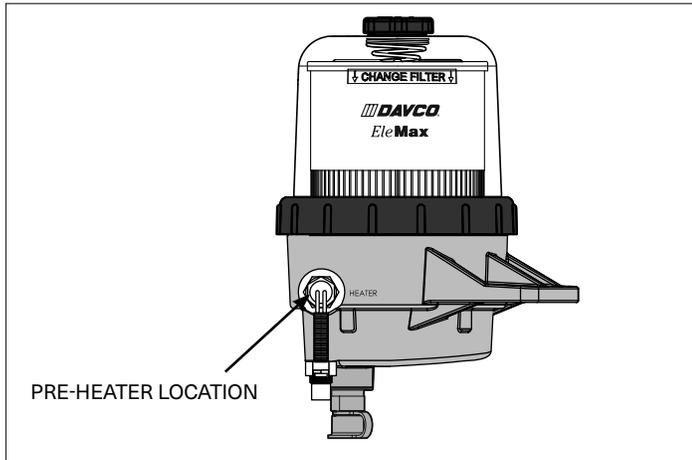
1. Remove the vent cap. Open the drain valve. Drain the Fuel Pro completely. Close the drain valve. The fuel can be reused after the installation.
