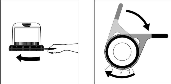
11. Prime the unit by filling the clear cover with clean diesel fuel until it reaches the top of the filter.
