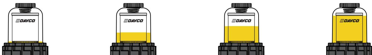
**When new, the fuel level in the filter will be very low with minimal restriction.** As the filter is used, contaminants collect on the filter from the bottom up. Fuel rises on the filter indicating remaining filter life.
